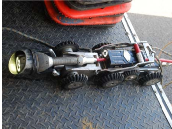
Figure 5-4. Side Sewer Inspection Camera.
